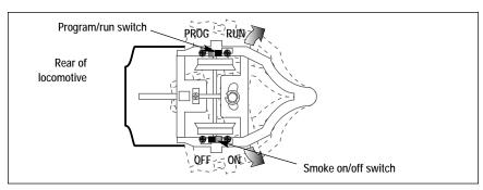
Figure 2. Locomotive switch locations
