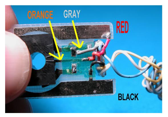
Here is the M-1 decoder installed. I left lengths of function wires in case I want to add a flashing warning beacon later.
