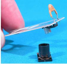
Remove all stock circuit board components on the bottom side. Don't forget that little tiny capacitor on the left!
